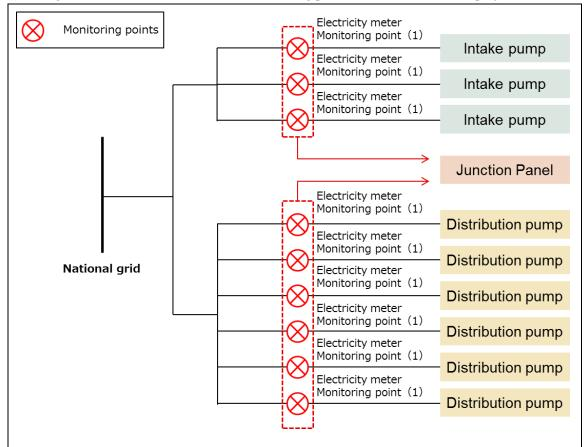
Electricity consumption of pumps is monitored by electricity meters as shown in the diagram above. The data monitored and required for verification and issuance are kept and archived for two years after the final issuance of credits.
