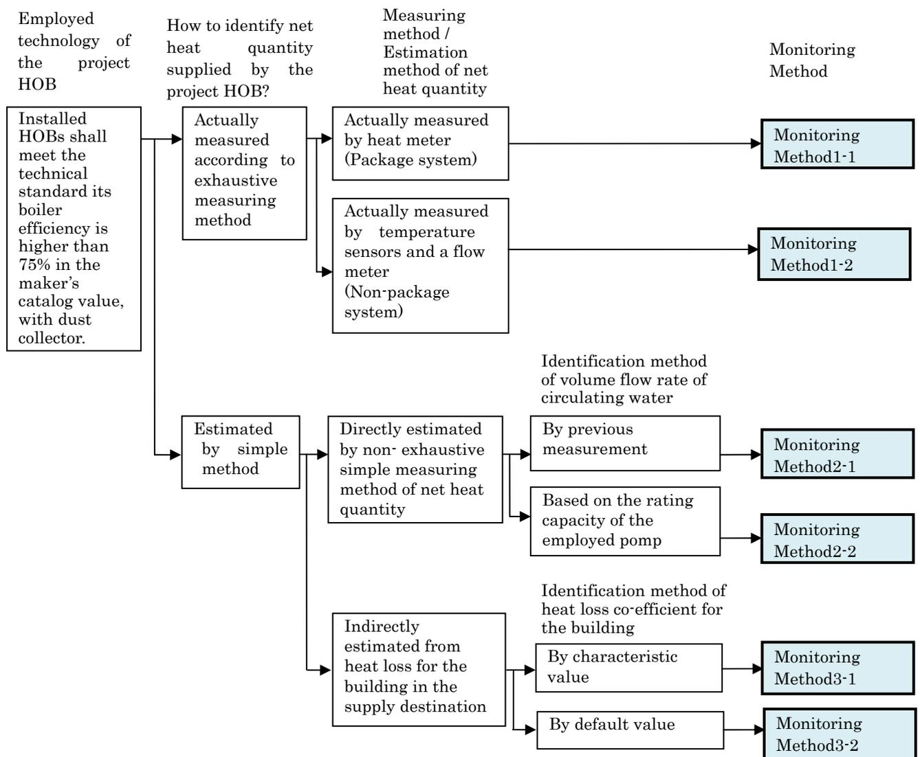
**Exhaustive measuring method of net heat quantity:** Method which measures directly net heat quantities of circulating water at inlet and outlet points of the water piping of the HOB, inserting temperature sensors into inside of the water piping. For measuring of water flow rate, the exclusive use water pipe which inside cross section area/or caliber is stereotyped in
