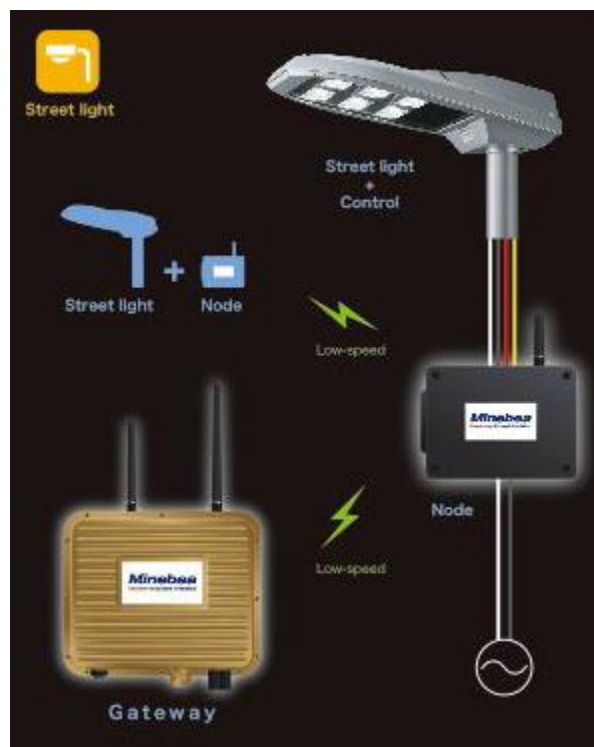
Figure 1: Image of LED street lighting system with wireless network control
