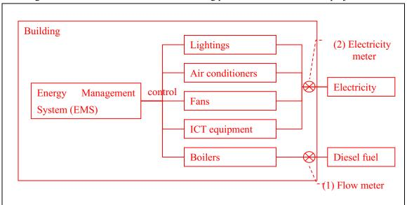
Please illustrate and describe all emission sources relevant to the project. Please also indicate all monitoring points for measurement\* with types of equipment to be installed for the proposed project in the figure. Each monitoring point for measurement should be indicated with monitoring point number(s) corresponding to the number of parameters listed in the Monitoring Plan Sheet.
