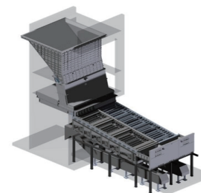
Waste to Energy Incinerator (Grate)
