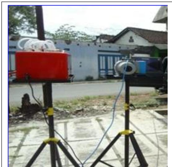
**Gambar 3.1.** Alat Ukur Udara Ambient: Gas Impinger (kiri) dan HVAS (High Volume Air Sampler, kanan)
